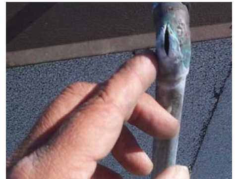
Split in water line leaking
